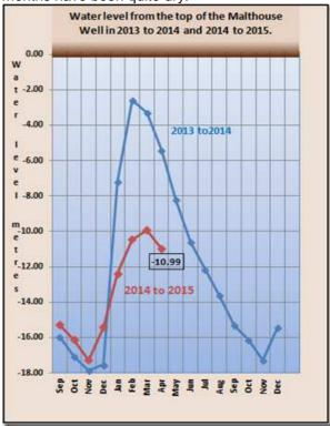
Groundwater levels in West Ilsley rise and fall with the seasons normally reaching a peak in the spring following replenishment through the late autumn and winter when losses by water evaporation and plant uptake are low. The Malthouse well is typical in this regard and in fact this year it peaked on 23rd March. Unless we get an exceptional period of rain the groundwater level should continue downwards through the summer and early autumn until the beginning of next winter.
